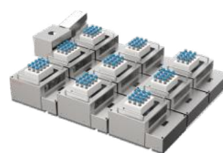
Up to 9 reaction shakers with temperature individually controlled, compatible with 8 mL and 40 mL reaction flasks; Integrated with an imaging module for high-resolution photos of the reaction system
